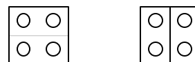
Figure 3. Partitioned cells. A horizontally partitioned cell on the left and a vertically partitioned cell on the right.
