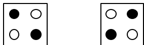
Figure 1. The schematic of a cell, with the two bi-stable states. The circles represent quantum dots. The circles filled in with black contain electrons. By convention, the left cell represents a logical zero, whereas the right cell represents a logical one.
